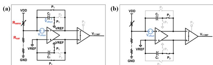
Fig. 2. Circuit operating of (a) P1 phase and (b) P2 phase
