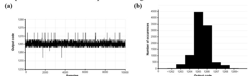
Fig. 7. Output (a) code variation and (b) histogram of 10000 samples
