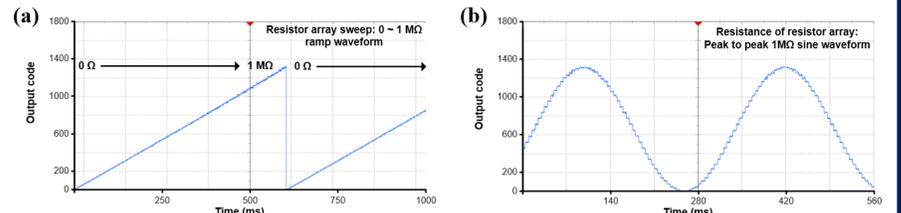
Fig. 6. Output code of sweeping the resistor (a) ramp and (b) sinusoidal form
